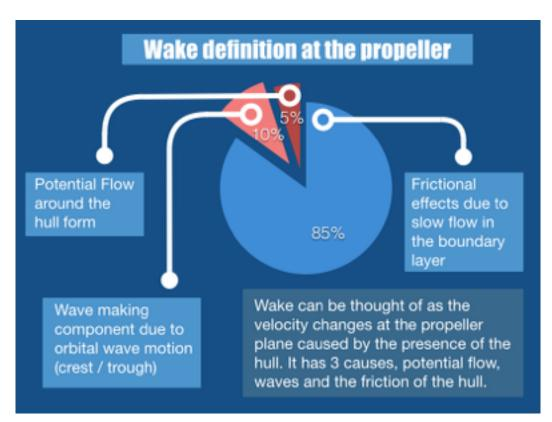
fraction. The wake is caused by 3 main factors, potential flow around the hull, friction of the hull and the waves the vessel makes. The contribution to the wake proportions on the chart to the left are for a typical vessel. In reality these depend upon the type of vessel and the speed of the vessel and several other factors.
