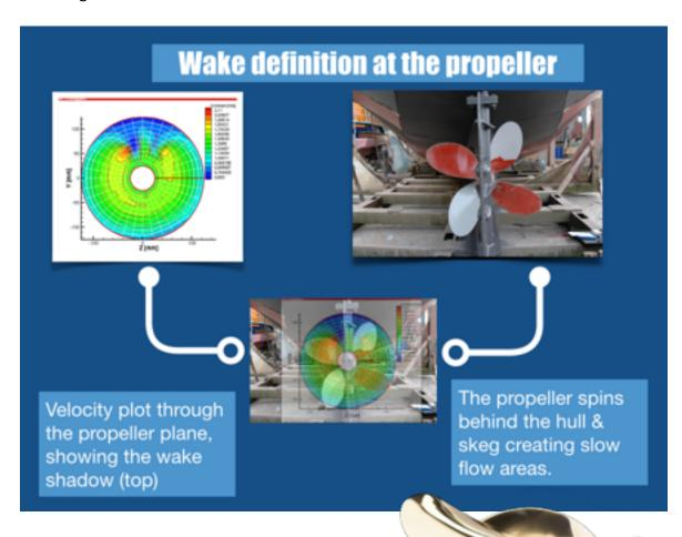
Putting this all together you get a velocity distribution at the propeller disc as shown above, the blue at the top is the slow flow and the green at the bottom is ambient flow.
